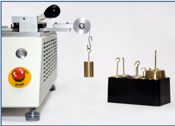
▲ Electronic calibration system using dead weights
